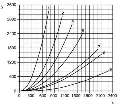
X- axis: Air Flow m³/h Y-axis: Pressure drop Pa
