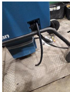
Hose fed to the unit clean side
