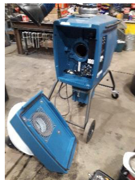
The fan / motor removed
