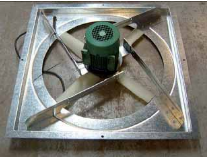
Reverse Air Cleaning Fan
