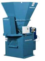
The integrated system crushes the chips, de-oils the chips and recovers
