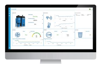
Nederman Insight is a cloud based IIoT\* platform designed specifically for filtration systems. It provides real time visualization and monitoring of system performance including customized dashboards and alarms.
