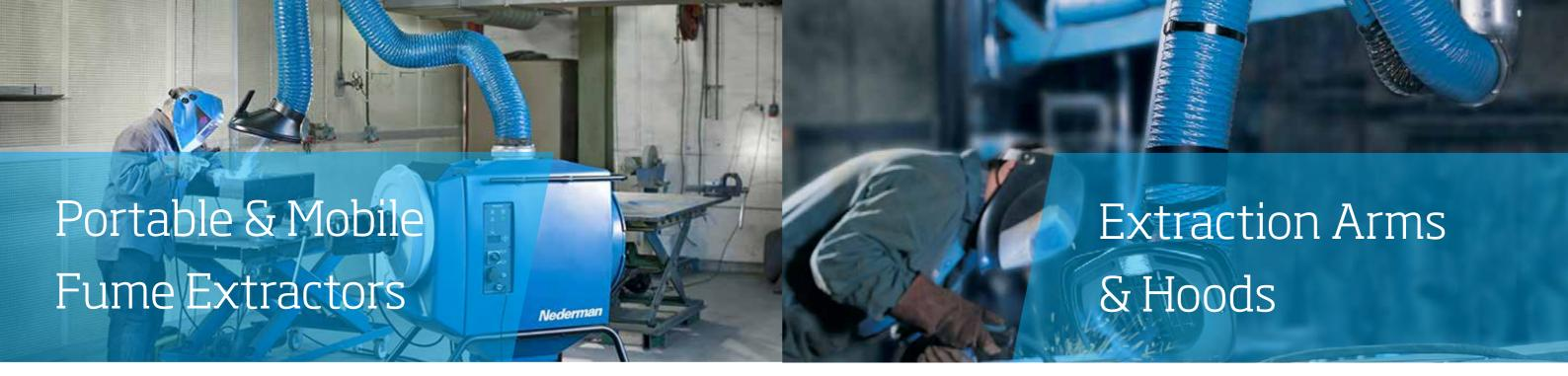
Mobile and portable fume extractors are common solutions that capture fume at the source with added flexibility to be moved around within workstations or factories to return clean air to the workplace. With their flexibility and variety of configurations, these solutions are excellent choices for both manual and automated welding cells.
