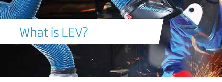
LEV or Local exhaust Ventilation is a means by which airborne substances are controlled and removed in order to prevent exposure to people in the workplace.
