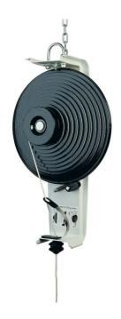
The balancer supports the tool or hose and keeps it lifted at all times. An integrated centrifugal brake prevents the balancer from recoiling too quickly, which minimizes the risk of personal injury and material damage. Hoist length, 8m (26 ft).
