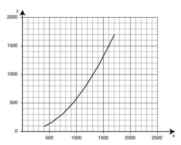
X: airflow, m³/h, Y: static pressure Pa
