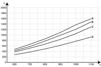
X: airflow m³/h, Y: static pressure Pa, A = 4 m horizontal, B =
