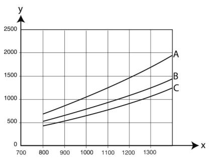
X: airflow, m³/h, Y: static pressure Pa,
