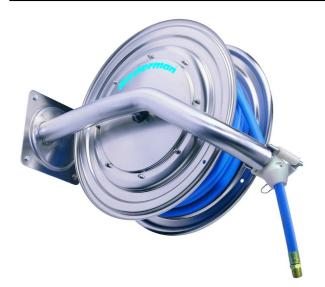
This stainless steel hose reel, made entirely of stainless steel, is designed specifically for the food processing industry. It is very easy to clean thanks to rounded edges and features an easy to dismantle hose outlet, an externally mounted swivel, and a minimum number of material joints.
