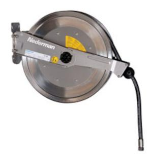
Series 889 Ex is a medium-sized hose reel for industrial use. All major components are made of stainless steel or electrically conductive composite material, required for chemically aggressive and explosive environments. The design of the reel makes it easy to keep clean for installation in areas with strict hygiene requirements. Approved for installation in ATEX zones 1, 2, 21 and 22 in accordance with ATEX2014/34/EC, Equipment group II, Category 2G D.
