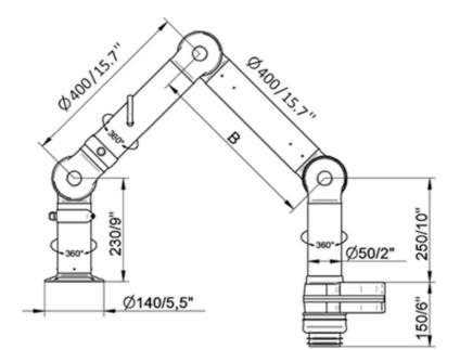
EK 2000 Arm(s): 1 x FX2 50 arm Hood(s): 1 x combination hood Hose: Ø 50 mm (2 inch), 3000 mm (118 inch) length Max. airflow: 100 m3/h (58.8 cfm)
