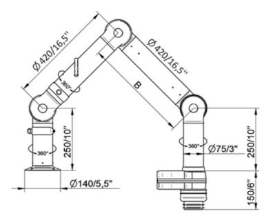
EK 3000 Arm(s): 1 x FX2 75 arm Hood(s): 1 x mini hood Hose: Ø 75 mm (3 inch), 3000 mm (118 inch) length Max. airflow: 150 m3/h (88.3 cfm)
