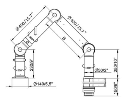
EK 2000 Arm(s): 1 x FX2 50 arm Hood(s): 1 x combination hood Hose: Ø 75 mm (3 inch), 3000 mm (118 inch) length Max. airflow: 100 m3/h (58.8 cfm)
