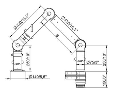
EK 3000 Arm(s): 1 x FX2 75 arm Hood(s): 1 x mini hood Hose: Ø 100 mm (4 inch), 3000 mm (118 inch) length Max. airflow: 150 m3/h (88.3 cfm)
