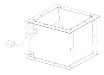
The damper type NFUS3 is used for emptying of material from the FM filters.
