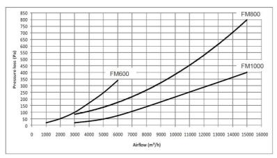
The curves indicate typical pressure drop across the silencers at different airflow volumes
