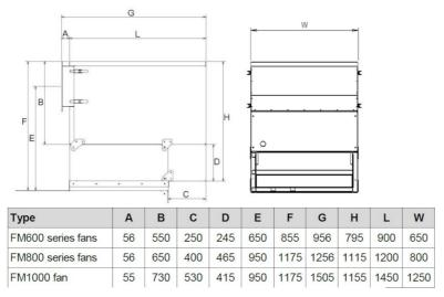
DUAL-Silencer dimensions (mm) with flanged outlet (for external duct connection)
