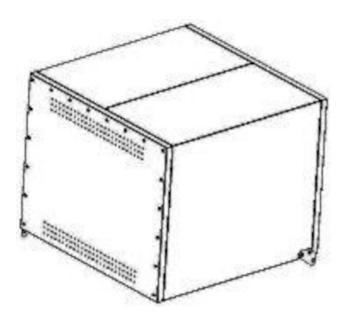
Both side panels with cooling air openings are de-mountable for access to the fan motor.
