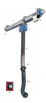
MagnaRail Green is a high capacity system designed to handle high operation requirements. Up to two vehicles can be attached to the same rail for a drive through or back in application for vehicles with low level tail pipes. The suction rail is formed in a configuration such that the extrusion serves not only as an exhaust duct, but also as the guide rail that the extraction trolley travels in. The rail is available up to 99 ft.
