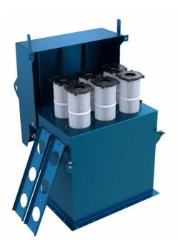
Specifically suited for use on silos that are pneumatically filled. The SiloSafe compact reverse jet tubular cartridge dust collector, available as a venting filter or with an integral fan, was developed specifically for silo and bin venting applications – incorporating Nederman UniClean (patented) cartridge technology for maximum cleaning efficiency and extended life.
