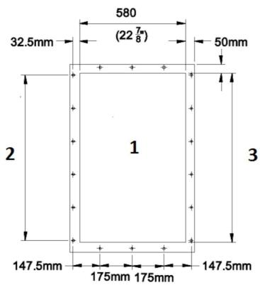
Filter mating Flange details: 1.18 Holes 12 dia. 2.5 pithces at 175 mm 3.1/Flange
