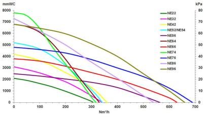
Air powered ejectors pressure / flow diagram
