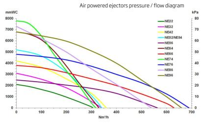
Air Powered ejectors
