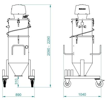
The height of the configuration is depending on filtermodule choosen.
