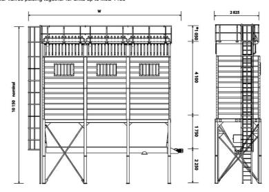
Hopper heights are typical values for  $55^\circ$  valley angle trough hopper
