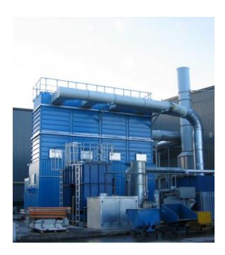
The MJB-G comprise an innovative range of robust, versatile tubular bag filter unit that build upon the experience of the well-established MJB bag filters.
