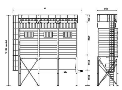
Hopper heights are typical values for  $55^\circ$  valley angle trough hopper
