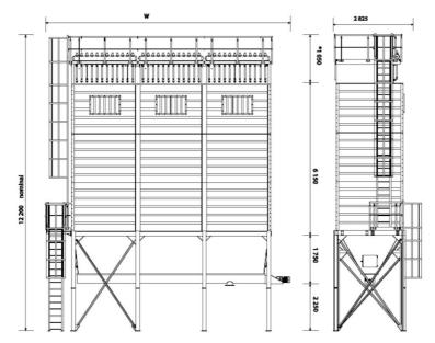
Hopper heights are typical values for  $55^\circ$  valley angle trough hopper
