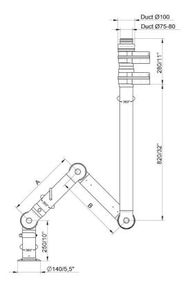
• FX2-CHEM-D75-L1100-Up-PLUS Part number: 70603244 Max. working radius: 1090 mm (42,9 in) A: 420 mm (16,5 in) B: 420 mm (16,5 in)
