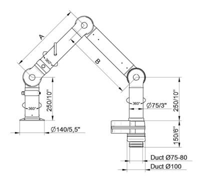
• FX2-CHEM-D75-L1100-Down-Low Part number: 70603344 Max. working radius: 1090 mm (42,9 in) A: 420 mm (16,5 in) B: 420 mm (16,5 in)
