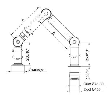
• FX2-CHEM-D75-L1100-Down-Through Part number: 70603444 Max. working radius: 1090 mm (42,9 in) A: 420 mm (16,5 in) B: 420 mm (16,5 in)
