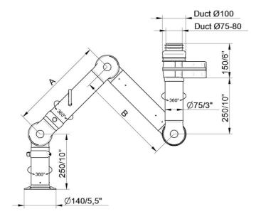
• FX2-CHEM-D75-L1100-Up-Low Part number: 70603144 Max. working radius: 1090 mm (42,9 in) A: 420 mm (16,5 in) B: 420 mm (16,5 in)
