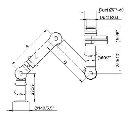
• FX2-ESD/EX-D50-L700-Up/Down-Low Part number: (70601244) Max. working radius: 630 mm (24,8 in) A: 400 mm (15,7 in)
