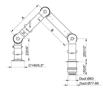
• FX2-ESD/EX-D50-L700-Up/Dow-Through Part number: 70601444 Max. working radius: 630 mm (24,8 in) A: 400 mm (15,7 in)
