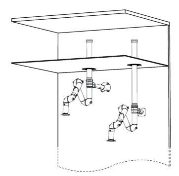
Wall mounting examples: Left: FX2-Up-Low arm with following accessories: -FX2-Bracket kit-D50/75/100-L500 -FX2-Ceiling cover plate-PLUS -FX2-Alu duct -FX2-Duct connector-ESD/EX-D75
