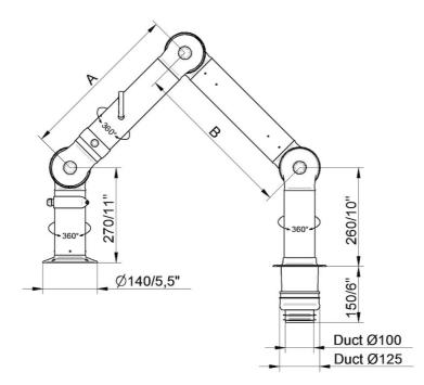
• FX2-CHEM-D100-L1200-Up/Down-Through Part number: 70605844 Max. working radius: 1170 mm (46,1 in) A: 450 mm (17,7 in) B: 450 mm (17,7 in)
