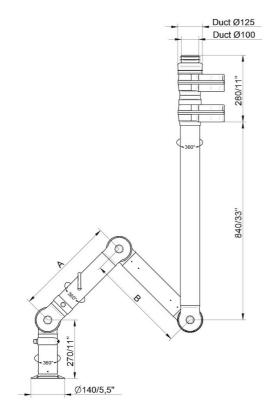
• FX2-CHEM-D100-L1200-Up-PLUS Part number: 70605744 Max. working radius: 1170 mm (46,1 in) A: 450 mm (17,7 in) B: 450 mm (17,7 in)
