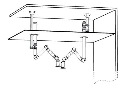
Ceiling mounting example: Left: FX2-Up-Low arm with following accessories: -FX-Classic bracket -FX-Cut2fit extension-L1100 -FX2-Alu duct-WHT -FX2-Duct connector-ORIG/CHEM-D100 -FX-Ceiling cover plate
