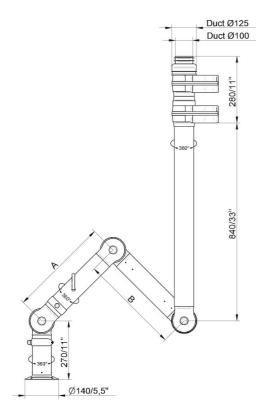
• FX2-CHEM-D100-L1200-Up-PLUS Part number: 70605744 Max. working radius: 1170 mm (46,1 in) A: 450 mm (17,7 in) B: 450 mm (17,7 in)
