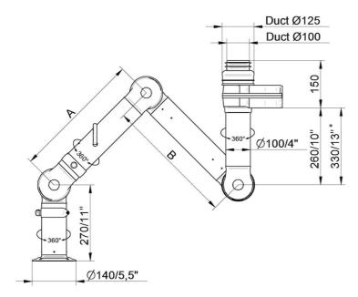
• FX2-CHEM-D100-L1200-Up/Down-Low Part number: 70605644 Max. working radius: 1170 mm (46,1 in) A: 450 mm (17,7 in) B: 450 mm (17,7 in)
