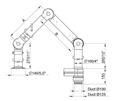
• FX2-CHEM-D100-L1200-Up/Down-Low Part number: 70605644 Max. working radius: 1170 mm (46,1 in) A: 450 mm (17,7 in) B: 450 mm (17,7 in)
