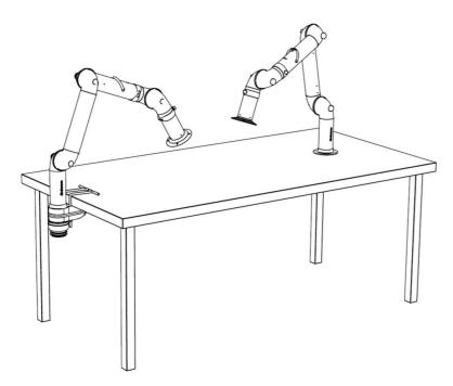
Bench mounting examples: Left: FX2-Down-Low arm with following accessories: -FX2-Bench bracket kit-D-50/75/100
