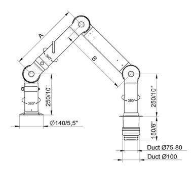
• FX2-ESD/EX-D75-L1100-Down-Through Part number: 70604244 Max. working radius: 1090 mm (42,9 in) A: 420 mm (16,5 in) B: 420 mm (16,5 in)
