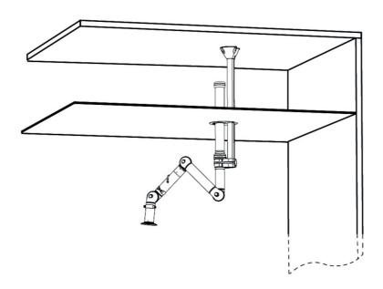
Ceiling mounting example: FX2-Up-Low arm with following accessories: -FX-Classic bracket -FX-Cut2fit extension-L1100 -FX2-Alu duct -FX2-Duct connector-ESD/EX-D100 -FX-Ceiling cover plate
