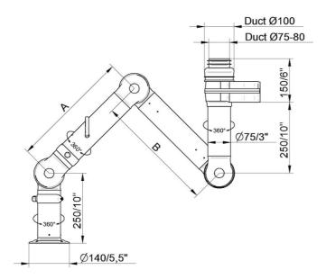
• FX2-ESD/EX-D75-L1100-Up-Low Part number: 70603944 Max. working radius: 1090 mm (42,9 in) A: 420 mm (16,5 in) B: 420 mm (16,5 in)
