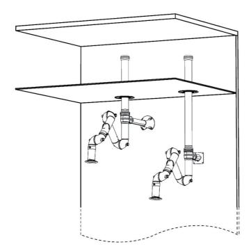
Wall mounting examples: Left: FX2-Up-Low arm with following accessories: -FX2-Bracket kit-D-50/75/100-L500 -FX2-Ceiling cover plate-PLUS -FX2-Alu duct -FX2-Duct connector-ESD/EX-D100
