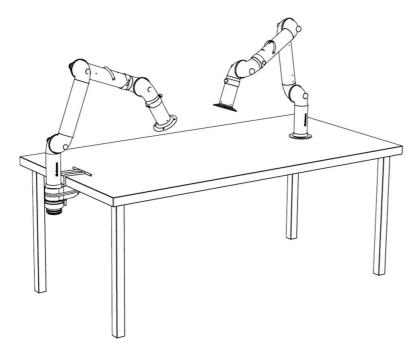
Bench mounting examples: Left: FX2-Down-Low arm with following accessories: -FX2-Bench bracket kit-D-50/75/100
