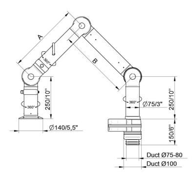
• FX2-ESD/EX-D75-L1100-Down-Low Part number: 70604144 Max. working radius: 1090 mm (42,9 in) A: 420 mm (16,5 in) B: 420 mm (16,5 in)
