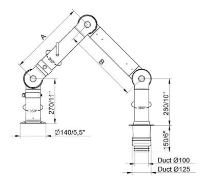
• FX2-ESD/EX-D100-L1200-Up/Down-Thru Part number: 70606744 Max. working radius: 1170 mm (46,1 in) A: 450 mm (17,7 in) B: 450 mm (17,7 in)
