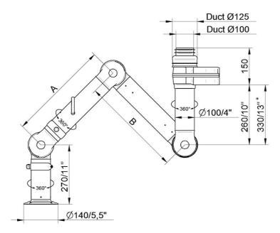
• FX2-ESD/EX-D100-L1200-Up/Down-Low Part number: 70606544 Max. working radius: 1170 mm (46,1 in) A: 450 mm (17,7 in) B: 450 mm (17,7 in)
