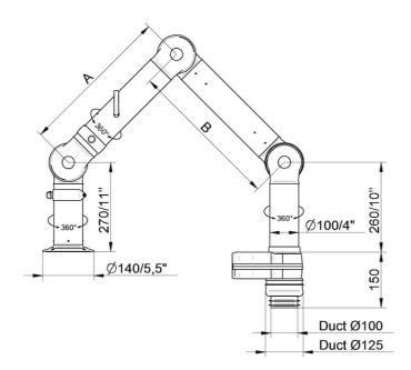
• FX2-ESD/EX-D100-L1200-Up/Down-Low Part number: 70606544 Max. working radius: 1170 mm (46,1 in) A: 450 mm (17,7 in) B: 450 mm (17,7 in)
