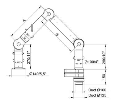
• FX2-ESD/EX-D100-L1200-Up/Down-Low Part number: 70606544 Max. working radius: 1170 mm (46,1 in) A: 450 mm (17,7 in) B: 450 mm (17,7 in)
