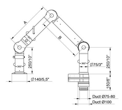
• FX2-ORIG-D75-L1100-Down-Low Part number: 70602544 Max. working radius: 1090 mm (42,9 in) A: 420 mm (16,5 in) B: 420 mm (16,5 in)
