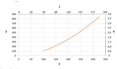
Pressure Drop diagram: 1) X- Axis: Air Flow Rate (cfm) 2) X- Axis: Air Flow Rate (m/h)
