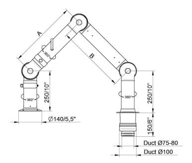
• FX2-ORIG-D75-L1100-Down-Through Part number: 70602644 Max. working radius: 1090 mm (42,9 in) A: 420 mm (16,5 in) B: 420 mm (16,5 in)
