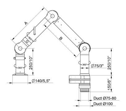
• FX2-ORIG-D75-L1100-Down-Low Part number: 70602544 Max. working radius: 1090 mm (42,9 in) A: 420 mm (16,5 in) B: 420 mm (16,5 in)
