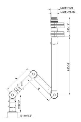
FX2-ORIG-D75-L1100-Up-PLUS Part number: 70602444 Max. working radius: 1090 mm (42,9 in) A: 420 mm (16,5 in) B: 420 mm (16,5 in)
