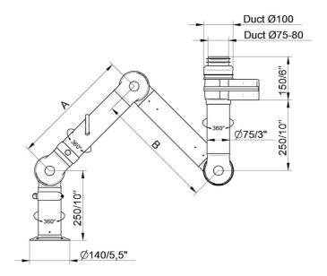
• FX2-ORIG-D75-L1100-Up-Low Part number: 70602344 Max. working radius: 1090 mm (42,9 in) A: 420 mm (16,5 inch) B: 420 mm (16,5 inch)
