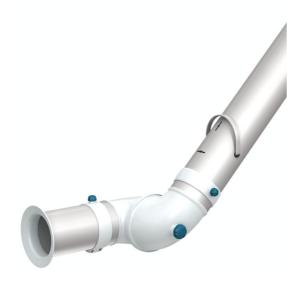
Nederman FX2 arms are made of lightweight anodized aluminium sections, with three adjustable, composite friction joints. Offering strength and durability combined with easy handling, they can be used in many types of environment. They are especially suitable for applications where small, flexible and easy-to-use arms are required
