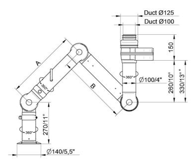
• FX2-ORIG-D100-L1200-Up/Down-Low Part number: 70604744 Max. working radius: 1170 mm (46,1 in) A: 450 mm (17,7 in) B: 450 mm (17,7 in)
