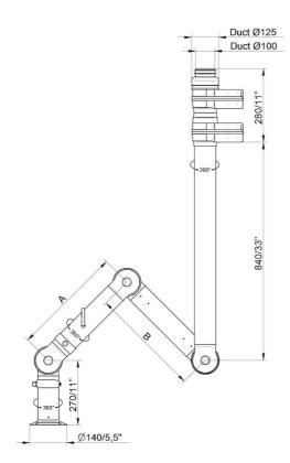
FX2-ORIG-D100-L1200-Up-PLUS Part number: 70604844 Max. working radius: 1170 mm (46,1 in) A: 450 mm (17,7 in) B: 450 mm (17,7 in)
