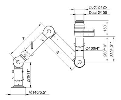
• FX2-ORIG-D100-L1200-Up/Down-Low Part number: 70604744 Max. working radius: 1170 mm (46,1 in) A: 450 mm (17,7 in) B: 450 mm (17,7 in)
