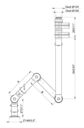
FX2-ORIG-D100-L1200-Up-PLUS Part number: 70604844 Max. working radius: 1170 mm (46,1 in) A: 450 mm (17,7 in) B: 450 mm (17,7 in)
