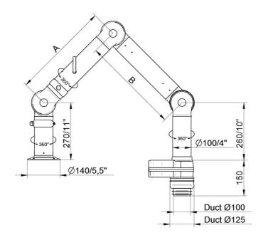
• FX2-ORIG-D100-L1200-Up/Down-Low Part number: 70604744 Max. working radius: 1170 mm (46,1 in) A: 450 mm (17,7 in) B: 450 mm (17,7 in)
