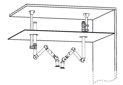
Ceiling mounting example: Left: FX2-Up-Low arm with following accessories: -FX-Classic bracket -FX-Cut2fit extension-L1100 -FX2-Alu duct -FX2-Duct connector-ORIG/CHEM-D100 -FX-Ceiling cover plate
