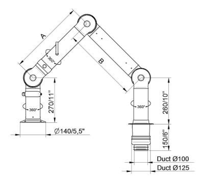
• FX2-ORIG-D100-L1200-Up/Down-Through Part number: 70604944 Max. working radius: 1170 mm (46,1 in) A: 450 mm (17,7 in) B: 450 mm (17,7 in)
