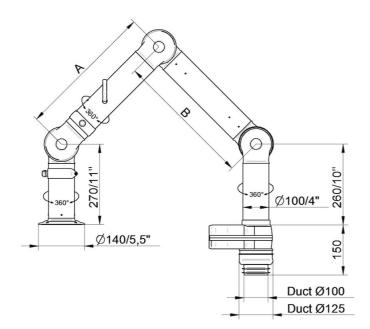
• FX2-ORIG-D100-L1200-Up/Down-Low Part number: 70604744 Max. rayon d'action: 1170 mm (46,1 in) A: 450 mm (17,7 in) B: 450 mm (17,7 in)
