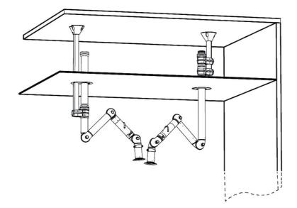
Ceiling mounting example: Left: FX2-Up-Low arm with following accessories: -FX-Classic bracket -FX-Cut2fit extension-L1100 -FX2-Alu duct -FX2-Duct connector-ORIG/CHEM-D75 -FX-Ceiling cover plate
