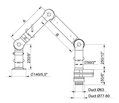
• FX2-ORIG-D50-L700-Up/Down-Low Part number: 70600144 Max. working radius: 630 mm (24,8 in) A: 400 mm (15,7 in)
