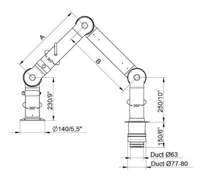
Part number: 70600344 Max. working radius: 630 mm (24,8 in) A: 400 mm (15,7 in) R: -
