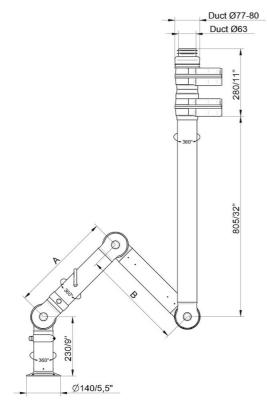
• FX2-ORIG-D50-L700-Up-PLUS Part number: 70600244 Max. working radius: 630 mm (24,8 inch) A: 400 mm (15,7 in)
