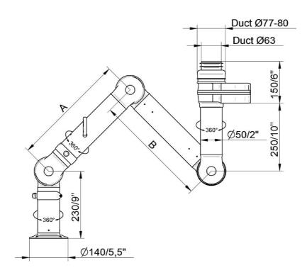
• FX2-ORIG-D50-L700-Up/Down-Low Part number: 70600144 Max. working radius: 630 mm (24,8 in) A: 400 mm (15,7 in)
