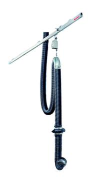
MagnaTrack ST is designed for stations with fewer runs. The freehanging exhaust hose is equipped with a swivel attached to a balancer, which moves on the guide track. A switch on the track separates the entire hose assembly from the vehicle in a one-step process, minimizing stress or strain from the vehicle to the exhaust hose or ceiling brackets. MagnaTrack ST is available in lengths from 6 to 12 m (20 to 40 ft) and it fits vehicles with low mounted exhaust pipes.
